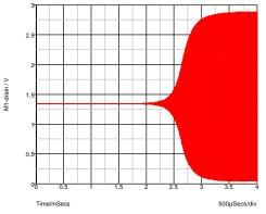
Figure 11-28: Start-up of a crystal oscillator.
