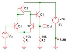
Fig. 2-1: A simple example for simulation, a bipolar buffer.
