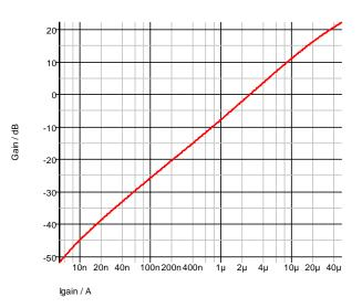
Fig. 10-8: Gain (in dB) vs. operating current (Igain).
