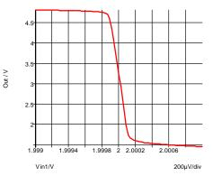
Fig. 4-13: Transfer curve for circuit in figure 4-12.
