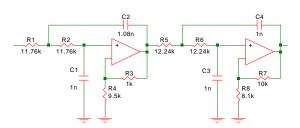
Fig. 13-12: 4th-order low-pass Butterworth filter in a voltage-controlled voltage-source design.
