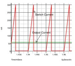
Fig. 14-25: Currents through switch and load.
