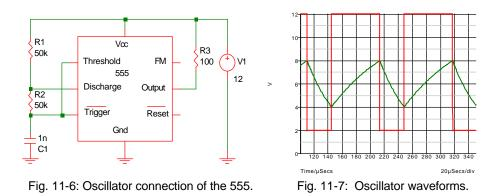
In the oscillator connection there are two external resistors and the voltage across C1 moves between 1/3 Vcc and 2/3 Vcc with a frequency and duty cycle of:
