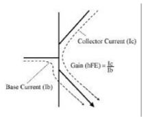
Fig. 1-3: The current flow and gain of an NPN transistor.
