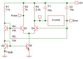
Fig. 11-29: Alternate crystal oscillator with bipolar devices.
