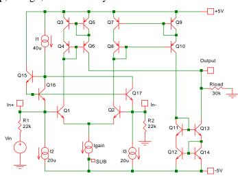
Fig. 10-2: An improved version of the bipolar transconductance amplifier with linearizing diodes.
