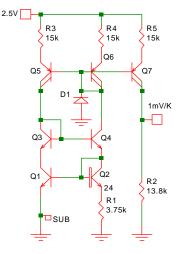
Fig. 16-21: Thermometer with Kelvin scale.
