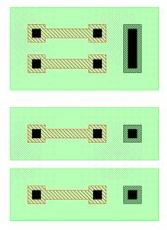
Fig. 17-10: Diffused resistors in a common (top) and in separate (bottom) islands.
