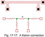
for a resistor and its equivalent circuit.
