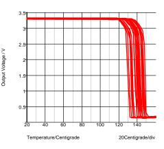
Fig. 14-6: Temperature shut-down.
