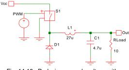
Fig. 14-19: Reducing a supply voltage with a series switch and inductor.
