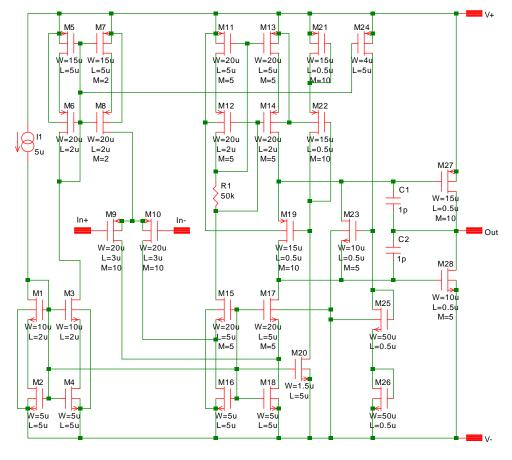
Fig. 8-21: Op-amp with P-channel input.
