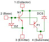
Fig. 2-11: Equivalent circuit for an integrated NPN transistor.
