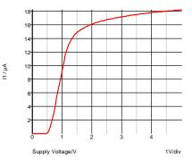
Fig. 5-3: I1 vs. supply voltage.
