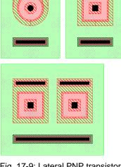
voltage). This field plate improves the gain of the transistor at low current by keeping p-type charges away from the surface. (In a CMOS process, the poly layer is used as a field plate, also connected to the emitter).
