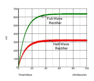
Fig. 16-20: Time constant and ripple for a one-pole low-pass filter used for averaging.
