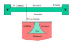
Fig. 10-25: Bulk or Epi-Pinch Resistor.
