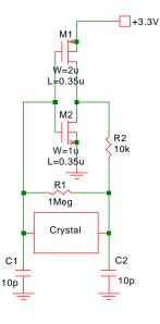
Fig. 11-26: Improved CMOS crystal oscillator.
