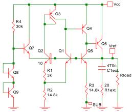
Fig. 7-5: Three terminal Brokaw reference with start-up.
