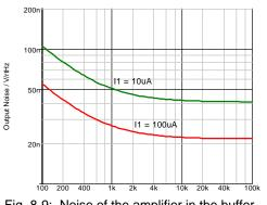
Fig. 8-9: Noise of the amplifier in the buffer connection.
