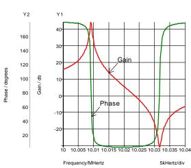
Figure 11-25: Series and parallel resonance of a crystal.
