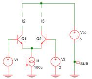
Fig. 4-1: In a differential pair a current is divided by two transistors.
