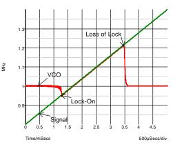
Fig. 12-6: Locking behavior of a phaselocked loop.
