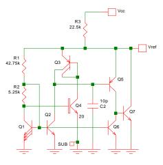
Fig. 7-18: A similar circuit, but with a single VBE (1.25V).
