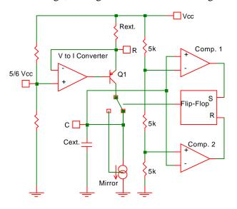
Fig. 11-1: The basic 566 Oscillator. In the actual circuit the comparators and the flip flop are combined in one Schmitt trigger.
