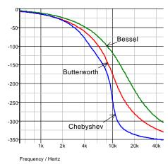
Fig. 13-9: Phase response of the three filters.
