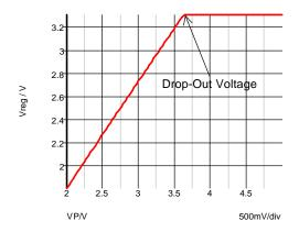
Fig. 14-10: Drop-out voltage at 20mA.
