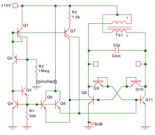
Fig. 11-21: Sine-wave oscillator with large amplitude.
