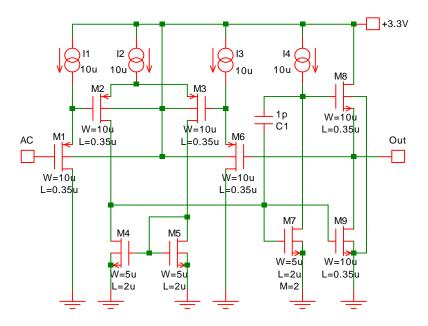
Fig. 16-18: CMOS half-wave rectifier with a single supply.
