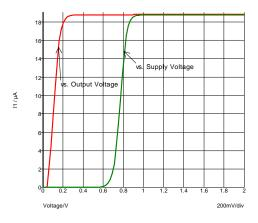
Fig. 5-15: Performance of the Erdi current source.
