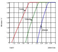
Fig. 14-12: Drop-out voltage.
