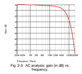
Our plot shows the output response of our buffer in the most simple AC analysis: a 1-Volt ac signal at the input on top of a DC Voltage of 2V, with the frequency swept from 200kHz to 200MHz. The output is in dB relative to the input, so 0dB is a "gain" of 1, -3dB is a "gain" of 0.708 (or a loss of 29.2%).
