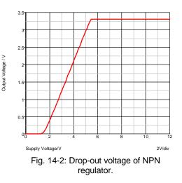
Watts, the regulator 4.36 Watts (with 12-Volts in), which is simply converted into heat. This the main disadvantage of a linear regulator. The heat is produced mainly by one device: Q13. Thus there will be a hot-spot on the chip and resulting temperature gradients, even with an adequate heat-sink. These temperature gradients are bound to influence other circuitry on the chip, including the regulator's own reference.
