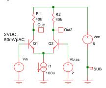
Fig. 4-7: A complete differential amplifier.
