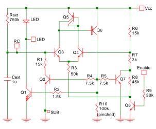
Fig. 11-15: Circuit generating brief current pulses.
