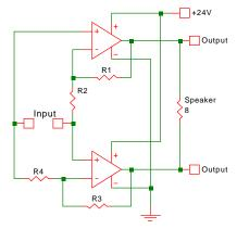
Fig. 14-33: Class AB amplifier with bridge output.
