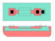
Fig. 1-24: Top view and crosssection of base-pinch resistor.
