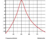
Fig. 13-17: Second-order band-pass filter response.
