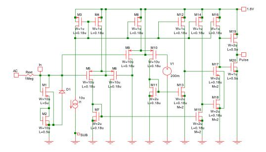
Fig. 16-27: CMOS version of zero-crossing detector.
