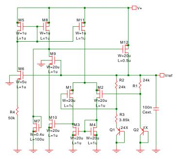
evaluation run. For this reason we will consider only a CMOS bandgap reference using substrate PNP transistors here. Q2 has a single (10um x 10um) emitter, O1 has 24 of them. Q2 is usually in the center, surrounded by 2 rows and columns of identical O1 devices. Get used to it: this pattern is very large
