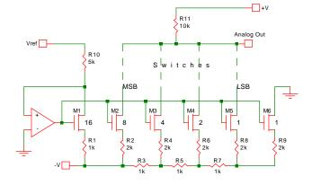
Fig. 15-7: CMOS current DAC with R-2R ladder.
