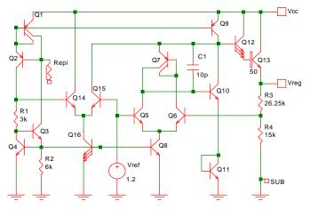
Fig. 14-1: Linear regulator with NPN power stage.
