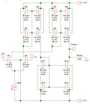
Fig. 10-5: A CMOS equivalent of figure 10-1.
