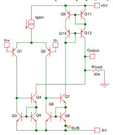
Fig. 10-1: A simple bipolar transconductance amplifier.
