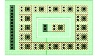
Fig. 17-6: 16:1 emitter ratio with epi-shift mismatch avoided.
