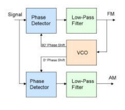
Fig. 12-7: Phase-locked loop with AM output.
