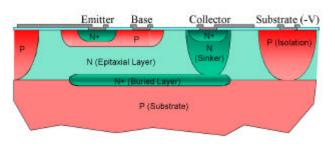
Fig. 1-10: A much improved planar, integrated NPN transistor. The buried layer and sinker lowers the collector resistance.
