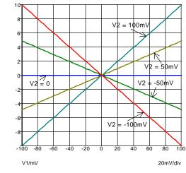
Fig. 16-7: Behavior of the four-quadrant multiplier.
