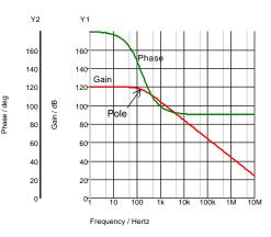
Fig. 6-9: Single-pole response. The phase never goes below 90 degrees.
