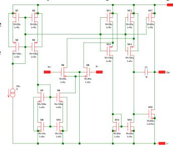
Fig. 8-16: Op-amp with folded-cascode input stage and a simple (and limited) output stage.
