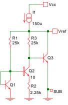
Fig. 7-3: Widlar's first bandgap reference.
