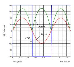
Fig. 12-2: With the VCO signal in-phase, the output is a rectified sine-wave with a positive average.
