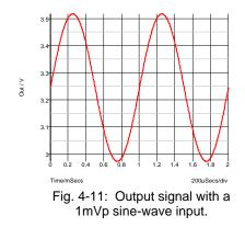
notice that there is a DC current flowing through R1. At the right end we connect it to a 3-Volt bias point, but at the left end the center of the sine-wave is not 3 but 3.25 Volts, i.e. we have a built-in offset. There are two reasons for this: 1. the two collectors of Q3 are not at the same potential and 2. the collector current of Q1 has to supply the base current for Q3.
