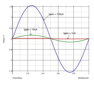
Fig. 10-4: Output waveforms (1kHz).
