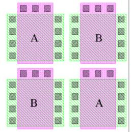
Fig. 17-14: A matching pair of n-channel transistors, using four devices.
