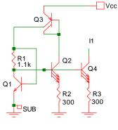
Fig. 5-12: Self-starting current source without large-value resistors.
