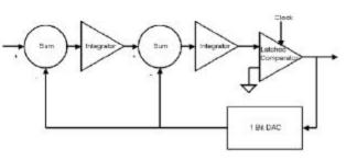
Fig. 15-13: Second-order Delta-Sigma ADC.
