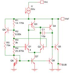
Fig. 7-14: Bandgap reference with curvature correction.
