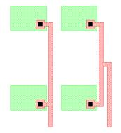
Fig. 17-18: Proper connection (on the right) for matching devices.
