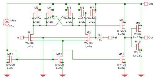
Fig. 9-5: CMOS comparator with hysteresis.
