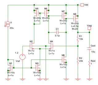
Fig. 14-11: Low-drop out CMOS regulator.
