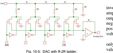
This is an inverting amplifier, so the output goes negative with a positive reference voltage. Using only two resistor values improves matching and trimming is
