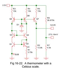
The centigrade (or Celsius) scale is the same as the Kelvin one, except for the zero set to 273.16K. So, all we need to do is to create an offset voltage of 273.16mV and read the temperature differentially.
