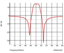
Fig. 13-19: Response of a fourth-order elliptic band-pass filter.
