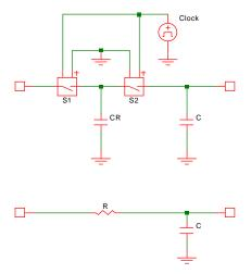
Fig.13-21: By using the equivalent resistance of a switched capacitor in a filter, only the capacitor ratio and the clock frequency are important.
