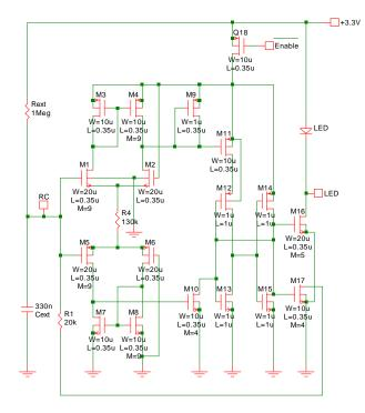
Fig. 11-17: CMOS design for a pulse generator. comparator (M1 to M4) sets the flipflop (M12 to M15); as it falls to 200mV above ground the lower comparator resets it. Cext is charged by Rext (1 second) and discharged by R1 (20msec). The two times are surprisingly accurate, exhibiting a 3% change from 3 to 3.6 Volts and 0 to 100°C.
