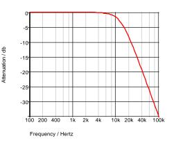
Fig. 13-6: Frequency response of the filter in figure 13-5.
