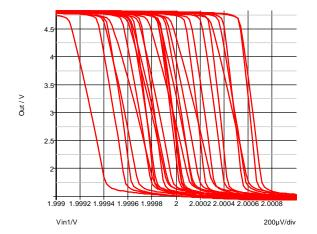
Fig. 4-14: Even a perfectly balanced differential amplifier (figure 4-12) has an offset voltage due to mismatch.
