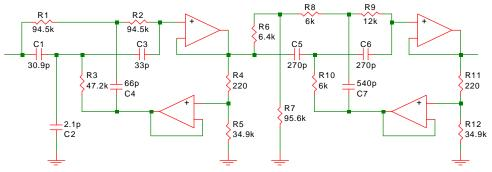
Fig. 13-18: A fourth-order, twin-T elliptic band-pass filter.
