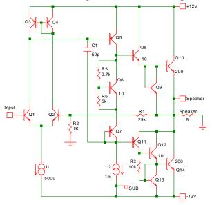
Fig. 14-29: 5-Watt bipolar class AB amplifier.
