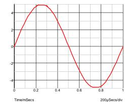
Figure 8-13: Output swing is limited by the saturation voltages of Q13 and Q14.
