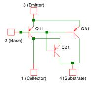
Fig. 2-12: Equivalent circuit for a lateral PNP transistor.
