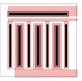
Fig. 17-7: NPN transistor for higher current.
