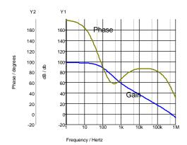
Fig. 14-8: Phase/gain diagram using three compensation capacitors.
