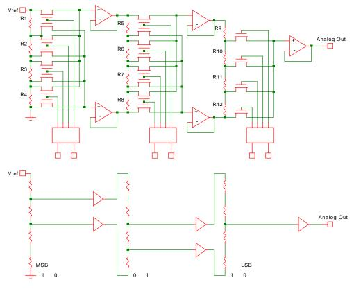
Fig. 15-3: 6-bit segmented DAC.
