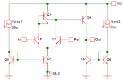
Fig. 9-1: Simple but accurate bipolar comparator.
