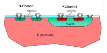
Fig. 1-18: Cross-section of an N-well CMOS process.
