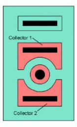
Fig. 1-17: A split-collector lateral PNP transistor.
