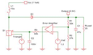
Fig. 14-26: Boost switching regulator.
