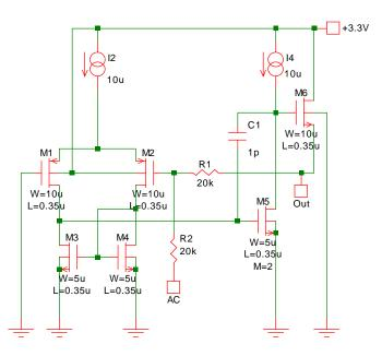
Fig. 16-19: Single-supply CMOS full-wave rectifier.
