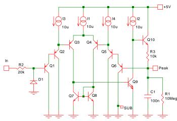
Fig. 16-11: Single-supply peak detector with a lower input current.
