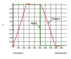
Fig. 8-5: Input and output waveforms for the buffer connection.
