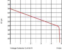
Fig. 3-4: Voltage dependence of I2.
