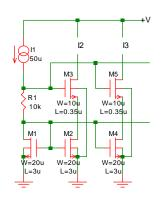
Here M3 and M5 simply shield M2 and M4 from changes in the output voltage. Their gates are held at a voltage slightly higher than the threshold voltage of M1 by causing a voltage drop in R1. In our case here this bias voltage is 500mV, which results in quite a remarkable
