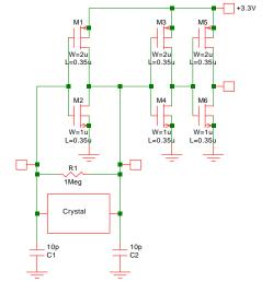
A crystal is simply a sliver of quartz that vibrates. Quartz is piezoelectric, i.e. a voltage applied
