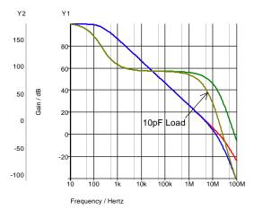
Fig. 8-17: Phase margin becomes critical with a capacitive load, unless the closed-loop gain is 40dB or larger.
