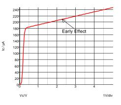
Fig. 1-11: Even with a constant base current the collector current increases with the collector-emitter voltage because the depletion layer narrows the base-width.
