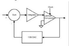
Fig. 15-11: Conventional diagram for a delta-sigma converter.
