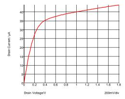
Fig. 1-20: Drain current vs. drain voltage with the gate voltage held constant.
