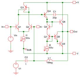
Fig. 6-14: Measuring gain and phase in a feedback loop.
