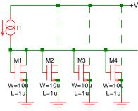
Fig. 3-19: Multiple current mirrors in MOS.
