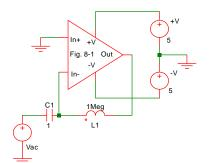
Fig. 8-2: Simulating loop gain and phase.
