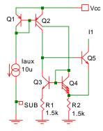
used to make a current source, let me point out that the accuracy of this current source is of no great importance. A bulk (epi) pinch resistor will do or any of the lesser current sources discussed above.
