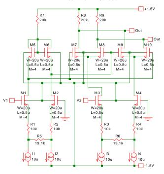
Fig. 16-9: Four-quadrant CMOS multiplier.
