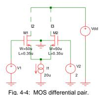
A differential pair using MOS transistors behaves almost identically, but *for entirely different reasons*. There is no dynamic emitter resistance; the gain is determined directly by the transconductance. This transconductance is also non-linear, increasing drastically with increasing gate voltage. Whereas in the bipolar transistor size is only of secondorder importance, transconductance in an MOS transistor is directly proportional to
