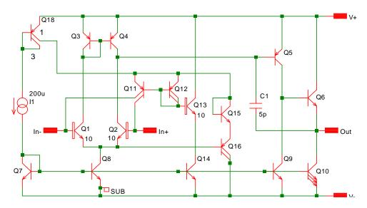
Fig. 8-15: Bipolar op-amp optimized for low noise.
