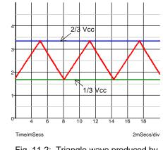
Fig. 11-2: Triangle-wave produced by the 566 oscillator.
