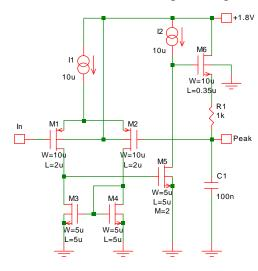
Fig. 16-12: CMOS peak detector.
