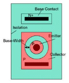
Fig. 1-16: The lateral PNP transistor.
