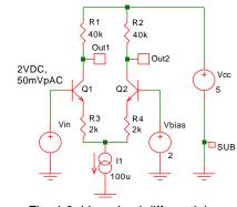
Fig. 4-8: Linearized differential amplifier
