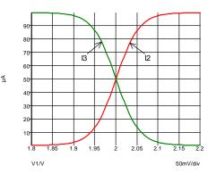
Fig. 4-2: The conversion from input voltage to current (the transconductance) is non-linear.....
