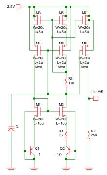
Fig. 16-23: CMOS Thermometer.
