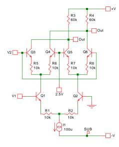
Fig. 16-6: Simple four-quadrant multiplier.
