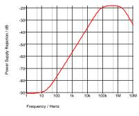
Fig. 14-18: ... which again impairs power supply rejection at high frequency.
