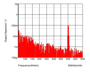
Fig. 14-46: Radiation spectrum across the load in figure 14-45.
