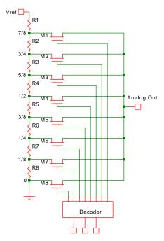
Fig. 15-1: 3-bit Divider DAC.
