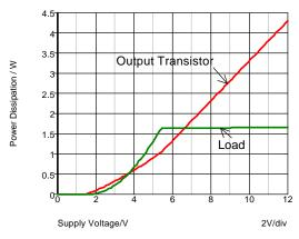
Fig. 14-3: In a linear regulator the energy not required by the load is converted into heat.
