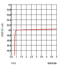
Fig. 3-13: Performance of the four-transistor current mirror.
