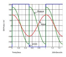
Fig. 12-3: With the phase of the VCO signal shifted by 90 degrees, the average of the output voltage is zero.
