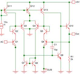
Fig. 16-14: Bipolar half-wave rectifier.
