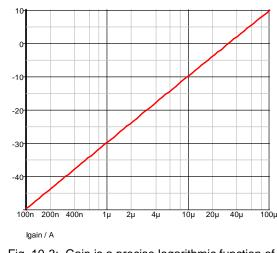
Fig. 10-3: Gain is a precise logarithmic function of Igain.
