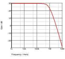
Fig. 14-30: Frequency response of the class AB amplifier.
