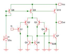
In figure 9-6 a Darlington input stage is used not to decrease the input current, but to allow the comparator to
