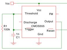
Fig. 11-10: 50% duty cycle oscillator.
