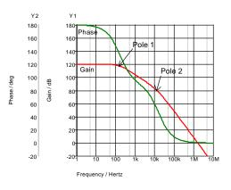
Fig. 6-10: Two poles in a feedback path approach zero degrees phase-shift.
