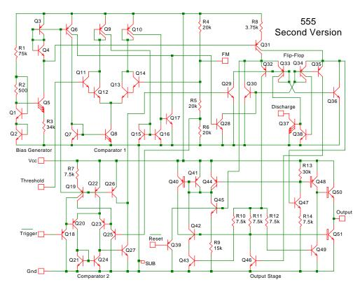
Fig. 11-8: An improved version of the 555 timer, 33 years after the original design.
