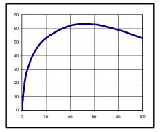
Figure 14-32: Power dissipation vs. power output in a class B amplifier.
