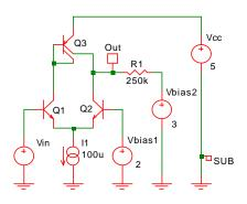
Fig. 4-10: Differential amplifier with an active load.
