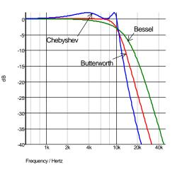
Fig. 13-8: Frequency responses of the three low-pass filters.
