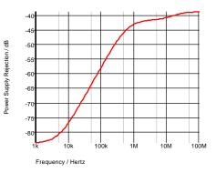
Fig. 14-14: ...but Rext limits power supply rejection at high frequency.
