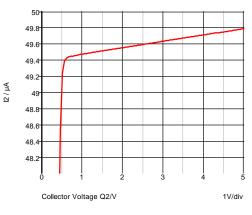
Fig. 3-8: Voltage dependence is now reduced to 0.7%.
