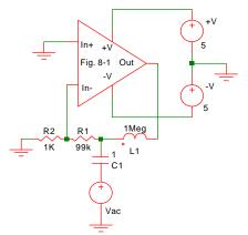
Fig. 8-6: Simulation of loop gain and phase with closed-loop gain of 100.
