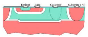
Fig. 1-15: At higher operating voltage the depletion regions around the NPN transistor become larger.
