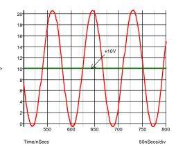
Fig. 11-22: The voltage swing of the oscillator extends to twice the supply voltage.
