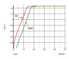
Fig. 7-11: Minimum operating current.
