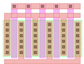
Fig. 17-13: Parallel connection of n-channel transistors.
