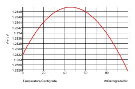
Fig. 7-6: Characteristic bow in the temperature curve of a bandgap reference.
