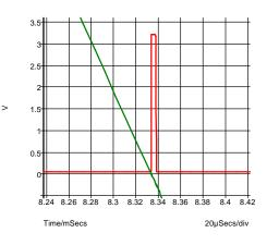
Fig. 16-26: AC slope and output pulse.
