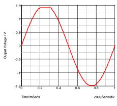
Fig 8-20: Output limits with 5kOhm load.
