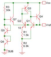
Four years after Widlar, Paul Brokaw published a paper entitled "A simple Three-Terminal IC Bandgap Reference". The core of the "Brokaw Cell" is formed by Q1, Q2, Q3, Q4, R1 and R2. (His actual circuit contained 14 transistors, so it wasn't so simple after all). The Brokaw cell needs a start-up circuit, which has been added here (Q7 lifts Vref to one VBE, which is sufficient for Q1 and Q2 to start drawing current).
