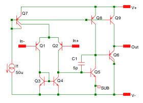
Fig. 8-10: PNP-input equivalent of figure 8-1.
