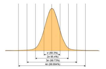
Fig. 2-8: The normal or Gaussian distribution.
