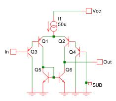
Fig. 4-17: A PNP Darlington input stage allows the input to move below ground.
