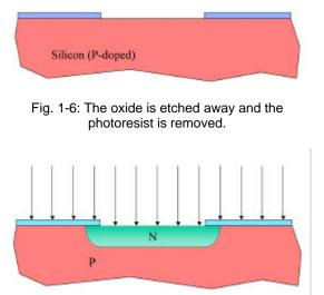
Fig. 1-7: A gas containing N-type dopants (boron, arsenic or antimony) diffuses slowly into the surface of the wafer at high temperature.
