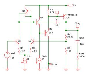
Fig. 14-15: Low drop-out regulator with external PNP transistor.
