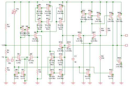
Fig. 12-9: Voltage-controlled oscillator with a Schmitt Trigger.
