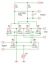
Fig. 12-1: The phase detector.
