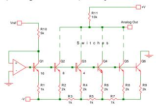
Fig. 15-6: Bipolar current DAC with R-2R ladder.
