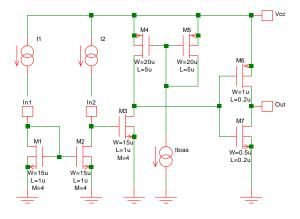
Fig. 9-9: CMOS version of current comparator.
