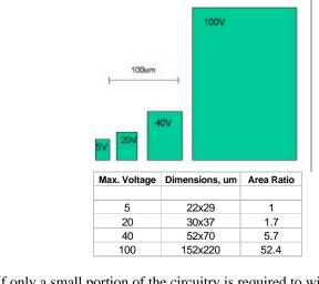
If only a small portion of the circuitry is required to withstand a high voltage, you wouldn't want *all* of the devices to pay the price of large dimensions. This then calls for a more complex process, one capable of producing both shallow and narrow devices and deep and wide ones.
