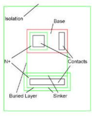
Fig. 17-1: Mask layers for an NPN transistor.
