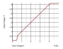
Fig. 2-2: A DC analysis, showing the common-mode range.
