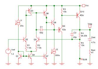
Output transistors need to be large to carry the current and thus have substantial capacitance, multiplied by the Miller effect. This forms an
