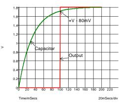
Fig. 11-20: Switching threshold of the 1.8V timer.
