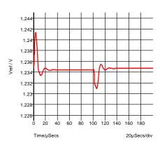
Fig. 7-8: Pulse response, indicating stability.
