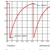
Fig. 11-18: Waveform at RC of figure 11-17.
