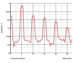
Fig. 6-3: Fast Fourier transform with low resolution.
