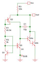
Fig. 7-17: A different design for a bandgap reference (2.5V).
