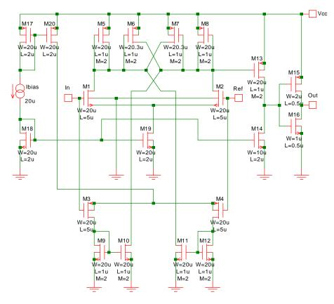
Fig. 9-7: CMOS comparator with rail-to-rail inputs
