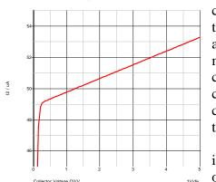
Fig. 3-2: The current of Q2 depends on its collector voltage.
