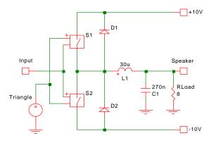
Fig. 14-41: Pulse-width modulated circuit with more practical component models. The diodes are now required to absorb the voltage spikes.
