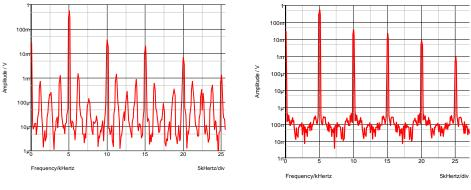
Fig. 6-4: Fast Fourier transform showing false peaks because of still insufficient resolution.
