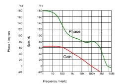
Fig. 14-17: Phase margin can only be kept high by a resistor in series with the output capacitor ....
