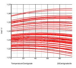
Fig. 7-7: In production (Monte Carlo analysis) you will see a larger deviation than merely the curvature.
