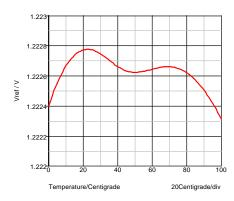
Fig. 7-15: The bow reduced by secondorder temperature compensation.
