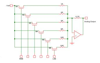
Fig. 15-4: DAC with binary weighted resistors.
