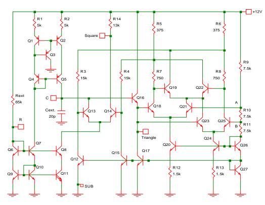
Fig. 11-11: A high-frequency triangle-wave generator.
