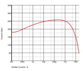
Fig. 1-12: The current gain (hFE) of a bipolar transistor drops off both at low and high currents.
