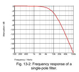
low-pass filter is said to have an attenuation of 20dB per decade or 6dB per octave (doubling of the frequency).
