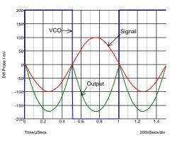
Fig. 12-4: At 180 degree phase shift the average of the output is negative.
