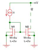
The current mirror also works with MOS devices, but it is not quite correct to call M1 a "diodeconnected transistor" (there is no "junction" diode).
