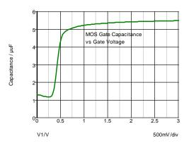
Fig: 1-26: The gate capacitance of an MOS transistor is greatly dependent on voltage.
