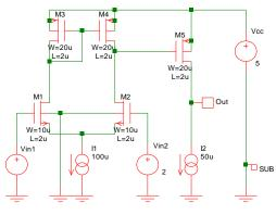
Fig. 4-15: Balanced CMOS differential amplifier.
