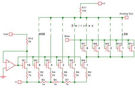
Fig. 15-8: Segmented current DAC.
