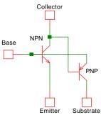
Fig. 1-14: When an NPN transistor saturates a stray PNP device leaks current to the substrate.
