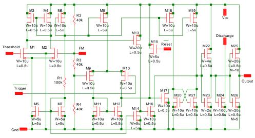
Fig. 11-9: A 5-Volt CMOS version of the 555 timer.
