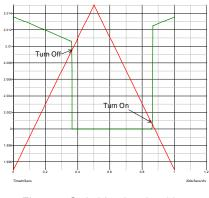
Fig. 9-4: Switching levels with hysteresis.
