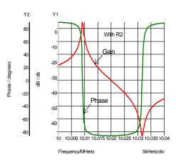
Figure 11-27: The insertion of R2 in figure 11-26 brings the phase shift to zero degrees at the series resonance.
