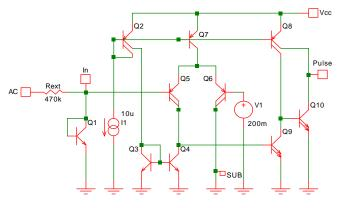
Fig. 16-25: Bipolar zero-crossing detector.
