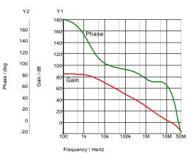
Fig. 8-3: For stable operation the gain of a loop must reach 0dB before the phase reaches 0 degrees.
