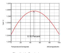
Fig. 7-12: Deviation over temperature (the bow.)
