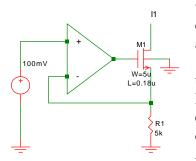
Fig. 5-18: Accurate current source with an op-amp and external resistor.
