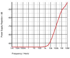
Fig. 14-9: Power supply rejection.
